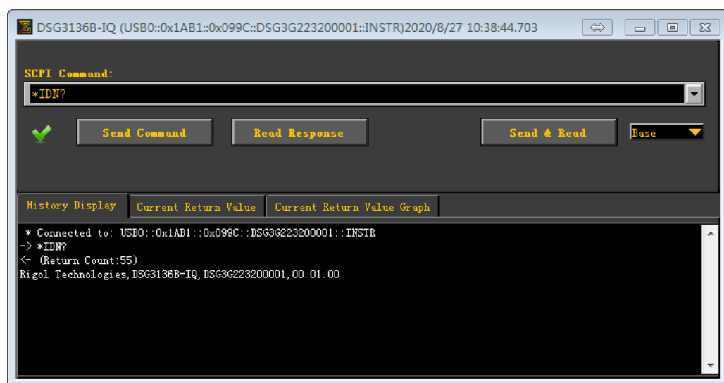
Figure 3-2 Read and Write Command via USB
